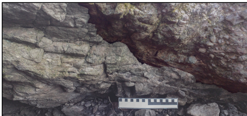
Figure 37. The breccia is clearly seen lying above the re-cemented quartzite, below which the quartzite is closely jointed, and easily eroded, producing a considerable undercut.
